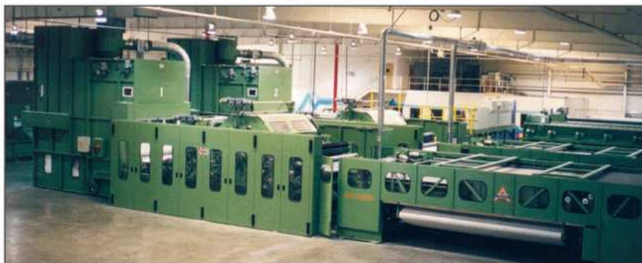
Compact CAV-4/10/16-DLL-D 棉胎生·的梳棉 Card for the production of waddings
