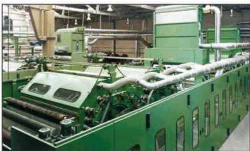
Compact TA-5/16-T-TA-5/16/16-DLL-D 地毯生产的特殊梳棉线 Special card for the production of carpets
